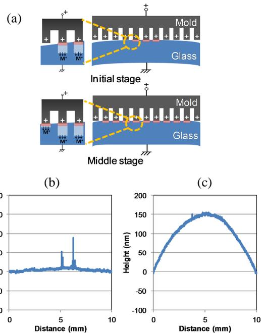
**Figure 2.** (a) Model of fine pattern formation by electrical nanoimprint. (b) and (c) are surface curvatures of mold substrate and soda-lime glass plate used for the imprint, respectively.
