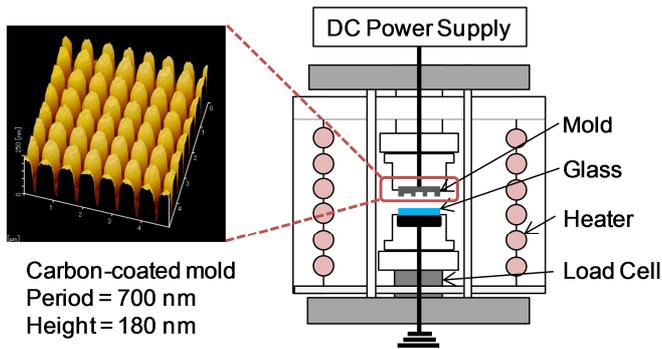
Figure 4. Experimental setup of electrical nanoimprint.
