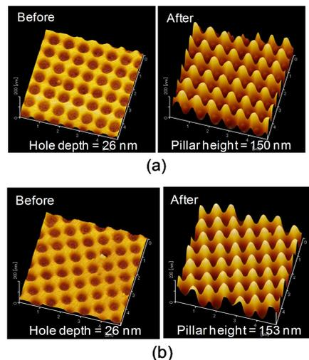
**Figure 3.** AFM views of glass plates imprinted under (a) 3 MPa and (b) 0.02 MPa, before and after KOH etching. Total charge estimated after electric imprint is 20.8 mC for (a) and 22.8 mC for (b).
