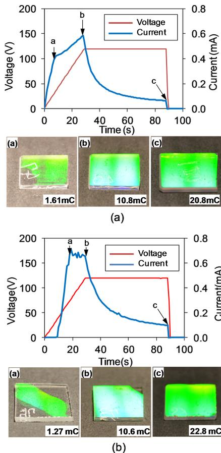
**Figure 1.** Time dependences of applied voltage and current (upper), and electrically imprinted glass surfaces (lower) at 450°C under the pressure of (a) 3 MPa and (b) 0.02 MPa. The specimen size is 10×10×1 mm.
